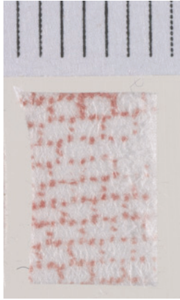
Figure 8. Transfer of water-soluble red dye onto test paper – scale marked in mm
