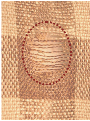
Figure 4. Brown-dyed homespun linen (circa 19th century), with weak and missing brown-dyed yarns (sample 11)
