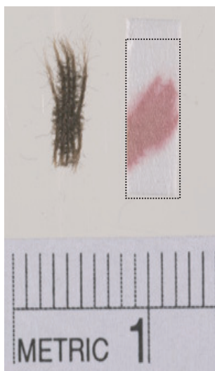
Figure 1. Positive iron test (outlined on strip) from severely deteriorated printed cotton textile fragment. Scale is in centimetres
