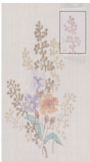
Figure 3. Positive iron test from printed cotton with no symptoms of damage. The shape of the dark brown printed area is mimicked in the magenta on the test strip (sample 8)
