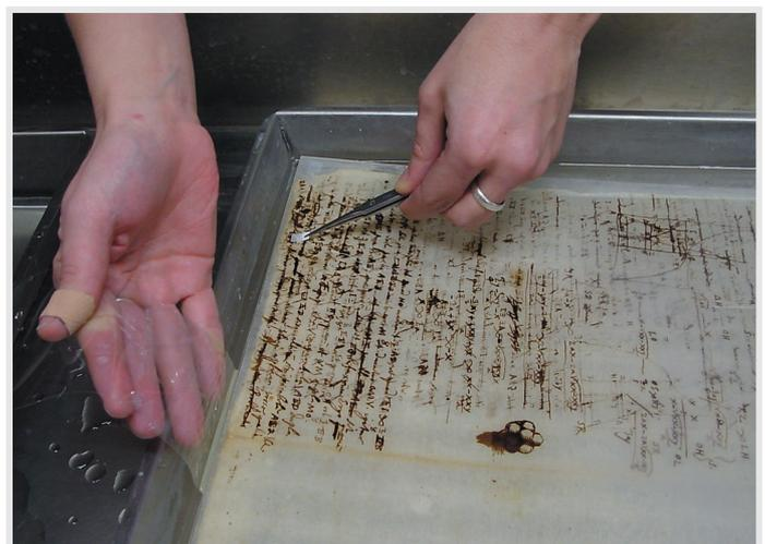
**8** Determination of iron ions on surfaces during treatment using a dry indicator paper..
