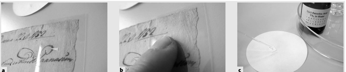
**6** Determination of iron ions on surface test strip covers half the ink, half the blank paper (a); gently press down the Melinex using a finger (b); a drop of ascorbic acid is added to the indicator paper (c).
